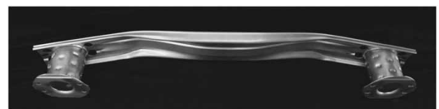
Fig. 9 Bumper system combining stay with beam
