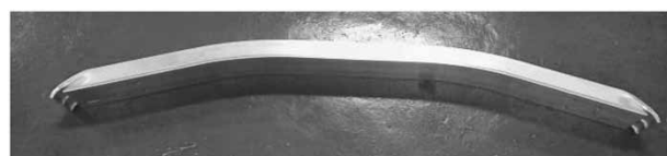
Fig. 6 Both-ends-formed bumper beam
