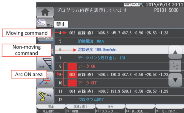
Fig.13 Coloring of robot teaching commands
