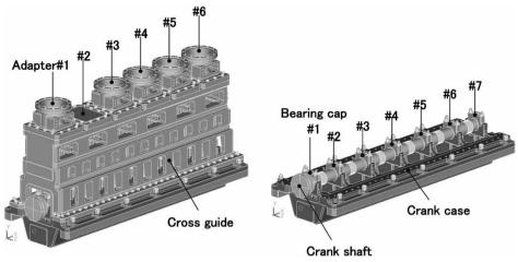
Fig. 4 3D-CAD model for FE analysis
