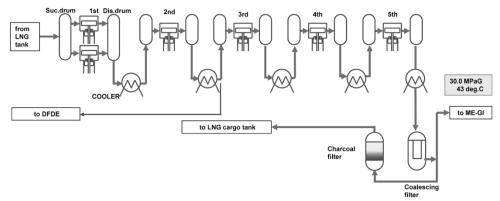
Fig. 2 ME-GI GIC flow diagram
