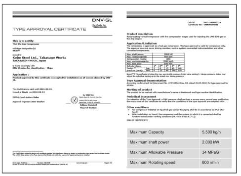
Fig. 5 Type approval certificate from DNV-GL
