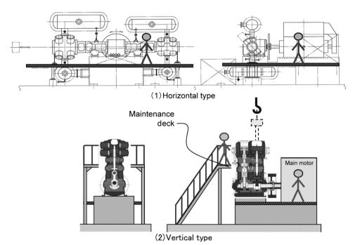
Fig. 3 Horizontal- and vertical-type reciprocating compressor units
