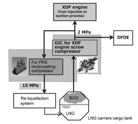
Fig. 6 Gas supply system for X-DF engine of LNG carrier
