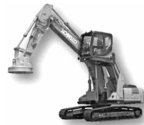
Fig.11 Overview of scrap handling machine with new-type magnet
