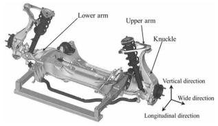
Fig. 4 Example of suspension members (front suspension structure of double wishbone type)<sup>8)</sup>
