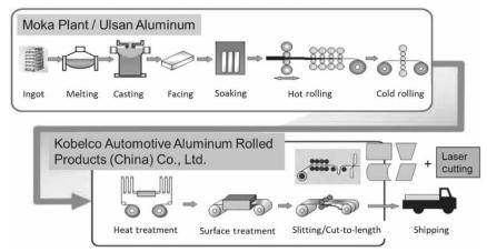
Fig. 3 Supply scheme of automotive aluminum sheet to China by Kobe steel group
