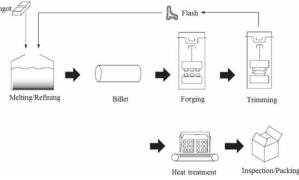
Fig. 5 Integrated production system for forged suspension of aluminum alloy in Kobe Steel 9)
