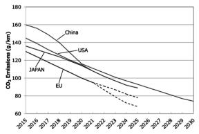
Fig. 1 Trends in strengthening of fuel efficiency and CO<sub>2</sub> criteria for passenger cars in Japan, Europe, China and the U.S.<sup>1</sup> (Fuel efficiency criteria converted to the amount of CO<sub>2</sub>)
