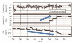
Fig.3 Transition of low coke rate operation
