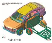
Fig.2 Simulation result of deformation of vehicle under side impact
