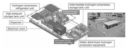
Fig. 2 Demonstration facility for refueling station of hydrogen based on renewable energy
