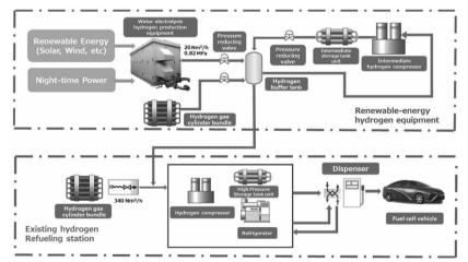
Fig. 1 Conceptual diagram of refueling station of hydrogen based on renewable energy
