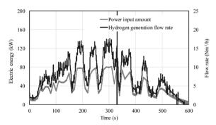
Fig. 4 Changes in electric energy and amount of hydrogen production over time (by pattern of cloudy weather in summer)
