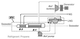
Fig. 5 Schematic diagram of process flow for LNG cryogenic power generation system (Rankine cycle)
