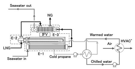
\*Heating, Ventilation, and Air Conditioning Fig. 7 Process flow of IFV for supplying cold energy to air conditioning apparatus
