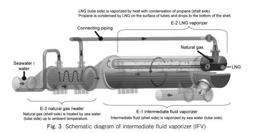
in an FSRU, it is suggested to use a non-flammable heat medium as an alternative.<sup>3)</sup>
