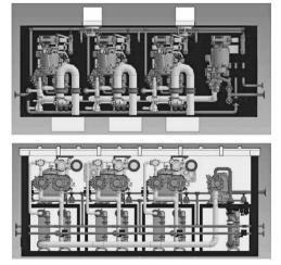
Fig.11 555 kW charging-cum-discharging unit
