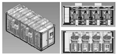
Fig. 6 500 kW discharging unit
