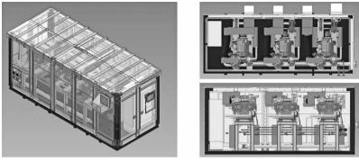
Fig. 5 500 kW charging unit
