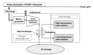
Fig. 2 Discharge flow of CAES system
