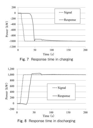
is launched to the maximum discharging state of 1 MW. In Fig. 7 and Fig. 8, zero on the vertical axis indicates the zero charging/discharging state, negative values indicate charging states (compressor operating states), and positive values indicate discharging states (expander operating state).
