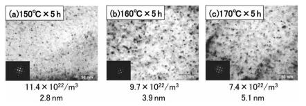
Fig. 5 TEM micrographs after pre-aging (upper values: number density of precipitates, lower values: size of precipitates)
