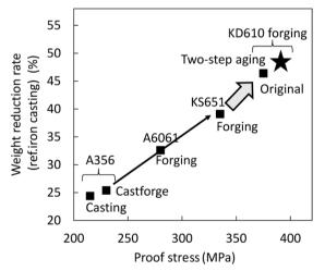
Fig.11 Relationship between proof strength and weight reduction rate of aluminum alloy<sup>8)</sup>
