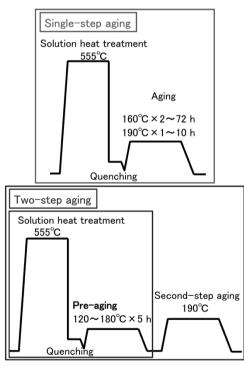
Fig. 1 Heat treatment processes of specimens
