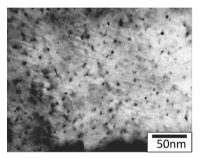
Fig. 9 TEM micrograph of specimen pre-aged at 160°C× 5 h and quenched at temperature of DSC peak 1 (Number density of precipitates: 5.2×10<sup>22</sup>/m<sup>3</sup>, size of precipitates: 6.7 nm)
