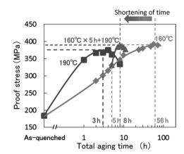
Fig. 3 Single-step aging curves at 160℃ and 190℃, and two-step aging curve at 190℃ after pre-aging at 160℃×5 h
