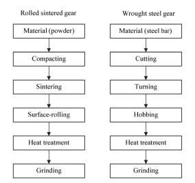
Fig. 4 Comparison of production process between rolled sintered gear and wrought steel gear
