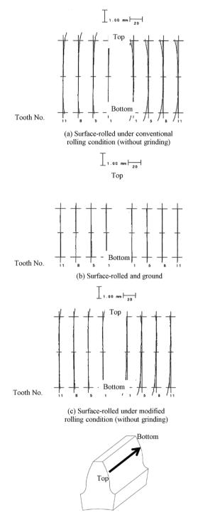
Fig. 6 Comparison of lead profiles
