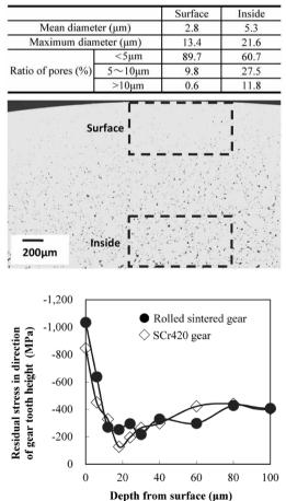
Fig. 3 Near-surface residual stress distribution in tooth depth direction
