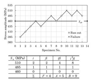
Fig. 6 Result of fatigue test using staircase method on developed steel
