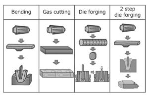
Fig. 2 Forging methods of crank throw
