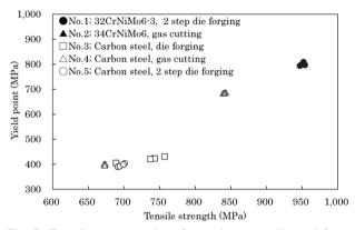
Fig. 5 Tensile test results of specimens collected from crank pin
