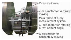
Fig.3 Photo of automatic X-ray system for measuring stress in fillet part of solidtype crank shaft
