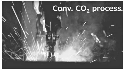
Conv. CO 2 process Wire feed rate : 16 m/min 350 A-37 V-500 mm/min
