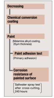
To reduce costs and environmental hazards, Kobe Steel also supplies galvanized steel sheet that has been chemical treated at the factory so that there is no need to prime the material before painting. In general, ZINKOBELLA (GX-GP treatment) and GALKOBE (Galvannealed) are most suitable for painting applications. For best results, choose a paint that is compatible with the chemical treatment applied.
