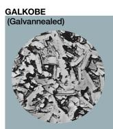
The alloying treatment diffuses iron particles in the coated surface to produce fine irregularities that ensure excellent paint adhesion.
