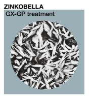
The phosphate film generated on the sheet surface assures outstanding paint adhesion, with an extremely smooth and attractive paint finish that only electrogalvanizing can provide.
