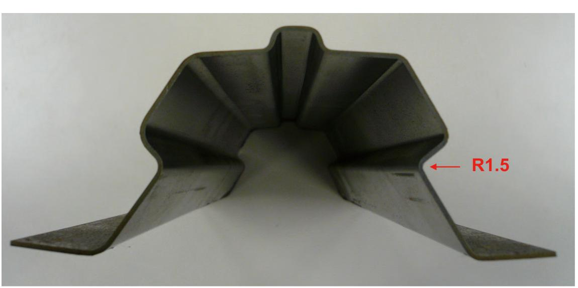
It can be bend to 1.5 R (1300 N/mm²-grade, 1500 N/mm²-grade, Thickness:1.2 mm)
