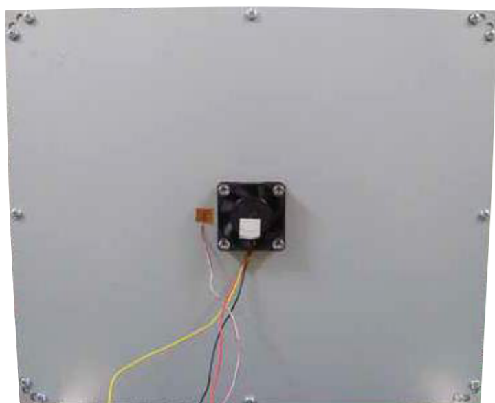
3 The fan is mounted on the EG lid
