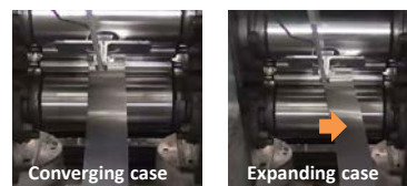
Experiment of lateral displacement using small scale test mill
