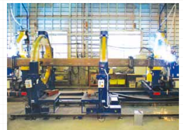
2-ARC welding joining HSS-column core
