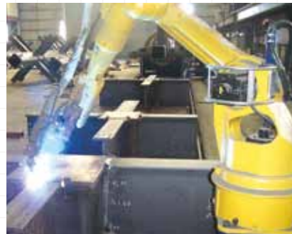
● Example of column large assembly system connection process
