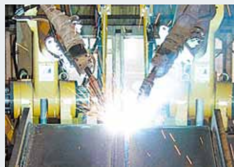
Central diaphragm is simultaneously welded.
