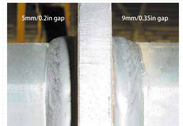
Effect on thin plate (effect on 2-ARC thin plate)
