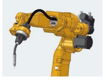
For the cable-integrated upper arm type, a wire feeder is mounted at the rear side of the upper arm; the torch cables extend from the wire feeder through the cable hole that runs alongside the upper arm. The torch body is supported at the wrist axis. .....
