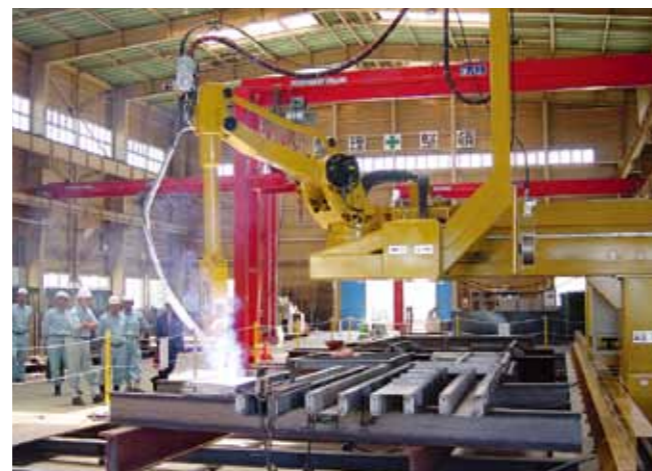
Figure 8: Compact and single robot welding system
