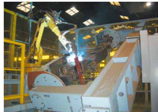
Figure 4: 2-3 meter long workpiece, held 1.5-2 meters above the floor level.
