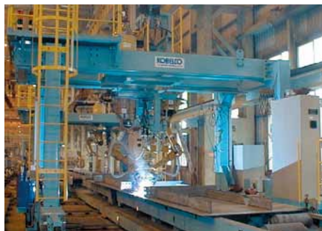
Figure 7: Gantry type twin welding system
