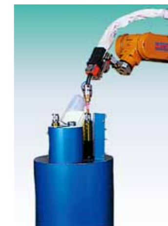
Figure 10: Automatic nozzle-changing device
