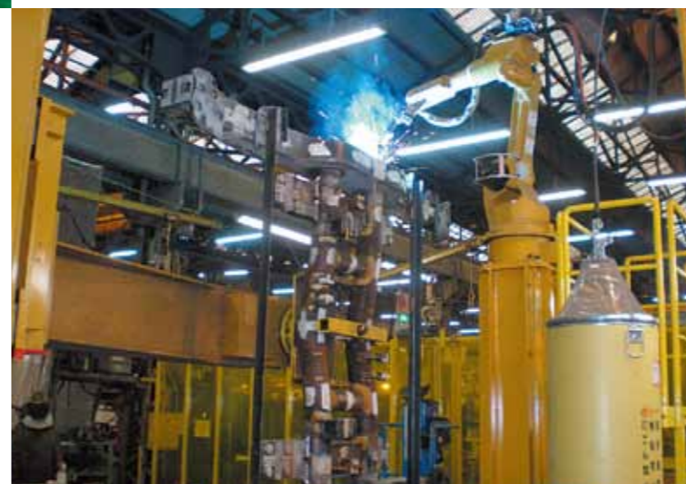
Figure 4: 2-3 meter long workpiece, held 1.5-2 meters above the floor level.
