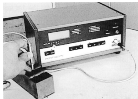
Fig. 3 — A Feritscope is most useful for measuring ferrite content of weld metals at site, because the probe is small enough to put on a small area of weld metal
