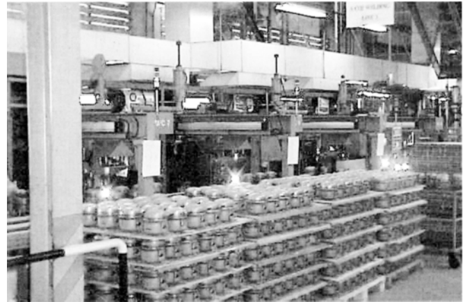
Fig. 1 — The welding process of refrigerator compressors involves CO 2 arc welding using automatic welding equipment
