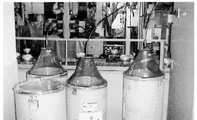
Fig. 2 — Kobelco ARROW Packs of MG-50 achieve consistently high quality welds, meeting MARIS's stringent requirements
