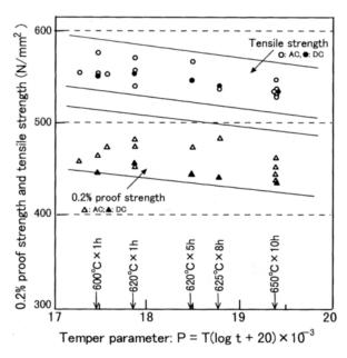
Fig. 3 — Effect of PWHT conditions on tensile properties of LB-52NS deposited metal
