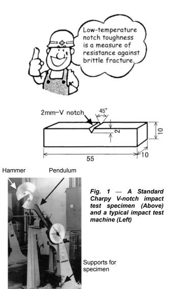
The most commonly reported result is the absorbed energy, but the percent shear fracture and the lateral expansion may also be reported. Typical transition temperature curves of carbon or low alloy weld metal are shown in Fig. 2.
