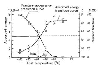
Fig. 2 — Typical transition temperature curves of a carbon or low alloy weld metal IS: shear, B: brittle)
