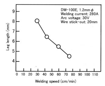
Fig. 4 — Leg length vs. welding speed in use of DW-100E in single pass horizontal fillet welding
