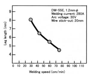
Fig. 4 — Fillet leg length vs. travel speed in use of DW-55E in single pass horizontal fillet welding
