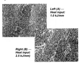
Fig. 2 — A comparison of microstructures of gas metal arc welded all-deposited metals of an ER80S-G trial wire, using two different amounts of heat input (X400) (Source: IIW Doc. XII-1647-00, 2000)
