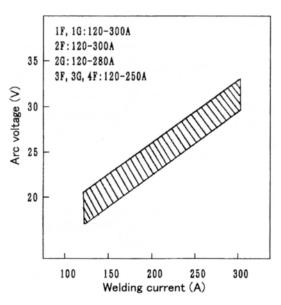
Fig. 3 — Proper ranges of welding currents and arc voltage (DW-55E, 1.2 mmØ); the welding positions of 2G, 3F, 3G and 4F restrict the use of high currents as shown in the figure respectively.
