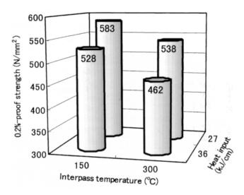
Fig. 3 — The effects of heat input and interpass temperature on 0.2%-proof strength of MG-60 all-deposited metal
