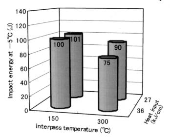
Fig. 5 — The effects of heat input and interpass temperature on Charpy impact energy (the average of 6 specimens) of MG-60 all- deposited metal
