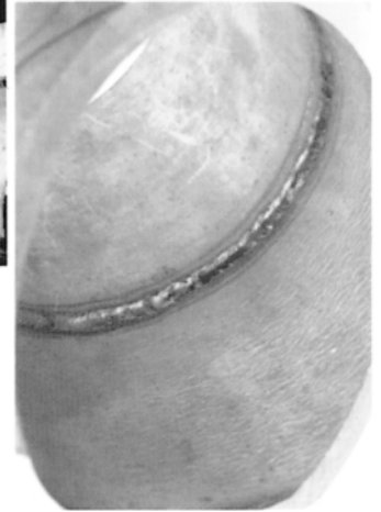
Figure 1. The reverse side of the root pass weld (right) made with a TGX-308L filler rod on a Type 304 pipe joint without back shielding.
