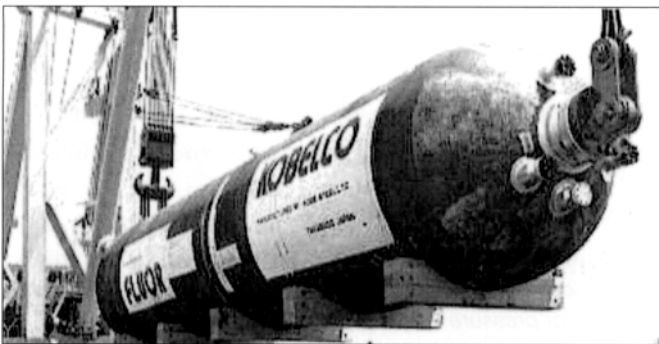
Fig. 1. Hydro-desulfurization reactor is a typical pressure vessel for which temper embrittlement resistance is strictly required.
