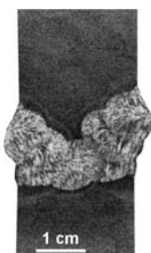
Figure 4: Macrostructure of an MF-33H/US-49 weld made in accordance with the welding conditions shown in Table 2.
