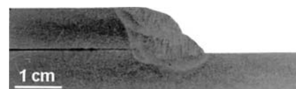
Figure 6: Macrostructure of a MF-300/US-36 weld made in accordance with the welding conditions shown in Table 5.
