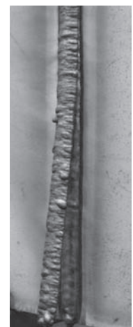
Figure 4: Self-peeling slag removal can save postweld cleaning time (Welding position: vertical)
