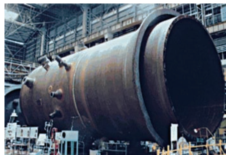
Reactor pressure vessels require an integrated manufacturing technique wherein base metals are matched with welding consumables of high and consistent quality.
