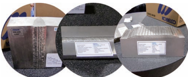
Bead samples of duplex stainless steel and Ni-based alloy weldments catch the eyes of visitors.
