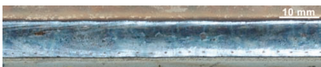
Figure 4: Schematic TRIFARC™ process and typical fillet weld bead appearance (Welding wire: FAMILIARC™ MX-200HS; 1.6 mmØ; Filler wire: FAMILIARC™ MG-1HS; 1.2 mmØ; Plate thickness: 12 mm; Welding speed: 2.0 m/min; Shop primer thickness: 30 µm).
