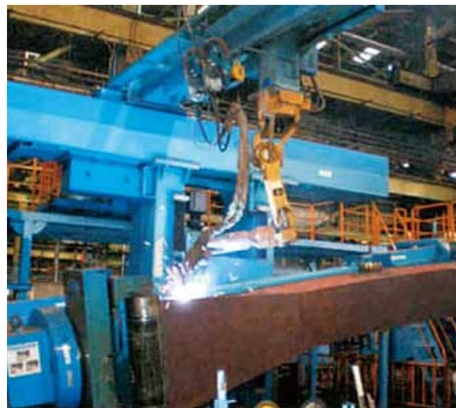
Figure 4: ARCMAN™-SR (suspended overhead) in operation on the boom in the tilted position.
