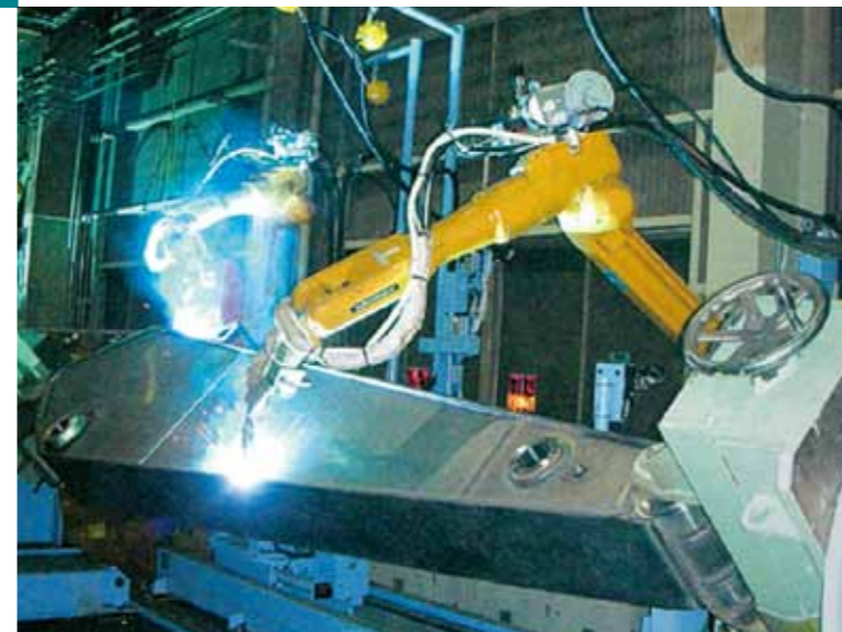
Figure 2: The twin-robot system reduces production time due to simultaneous operations.
