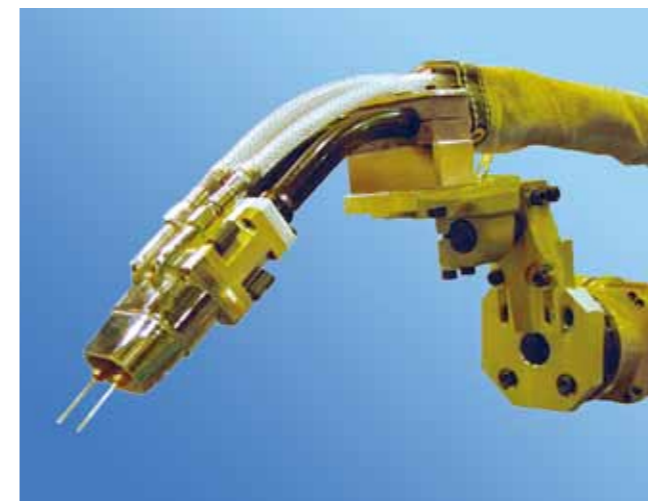
Figure 6: Compact integrated tandem torch offers easier access in a confined space and prevents the welding cable from getting tangled around the wrist of the robot.
