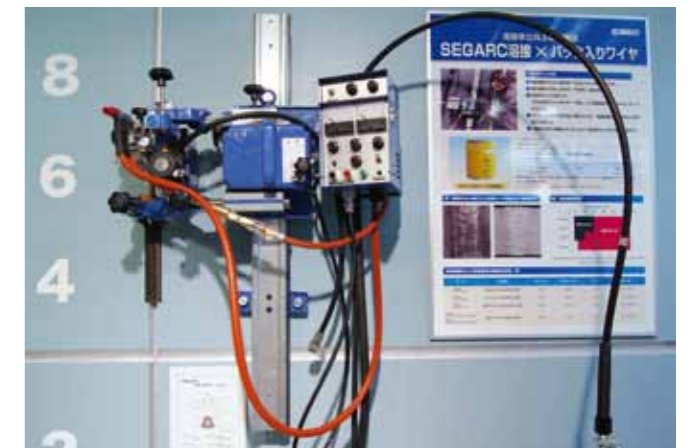
SEGARC™-2Z, an electrogas arc welding device, attached along the vertical butt joint of the simulated hull.
