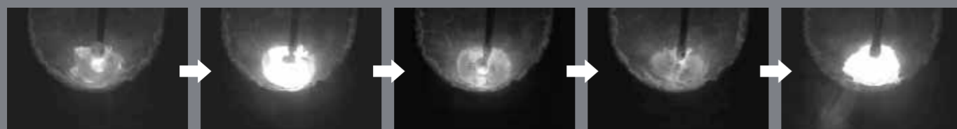
(1) droplet produced (2) droplet squeezed (3) current decreased (4) droplet detached (5) droplet produced.
