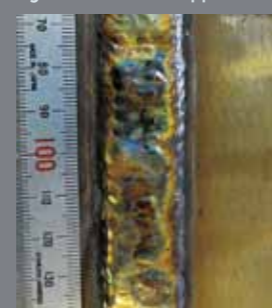
Figure 1: Weld bead appearance
