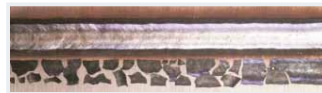
Figure 4 : Slag removability and bead appearance right after welding (DW-308L)
