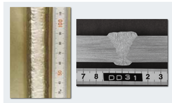
Figure 11 : Bead appearance and macrostructure by DW-2594 in 3G position. (80%Ar-20%CO 2 shielding, 160A-26V)
