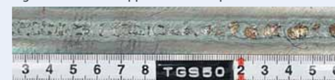
Figure 2: Back bead appearance in 1G position
