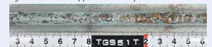
Figure 4: Back bead appearance in 1G position
