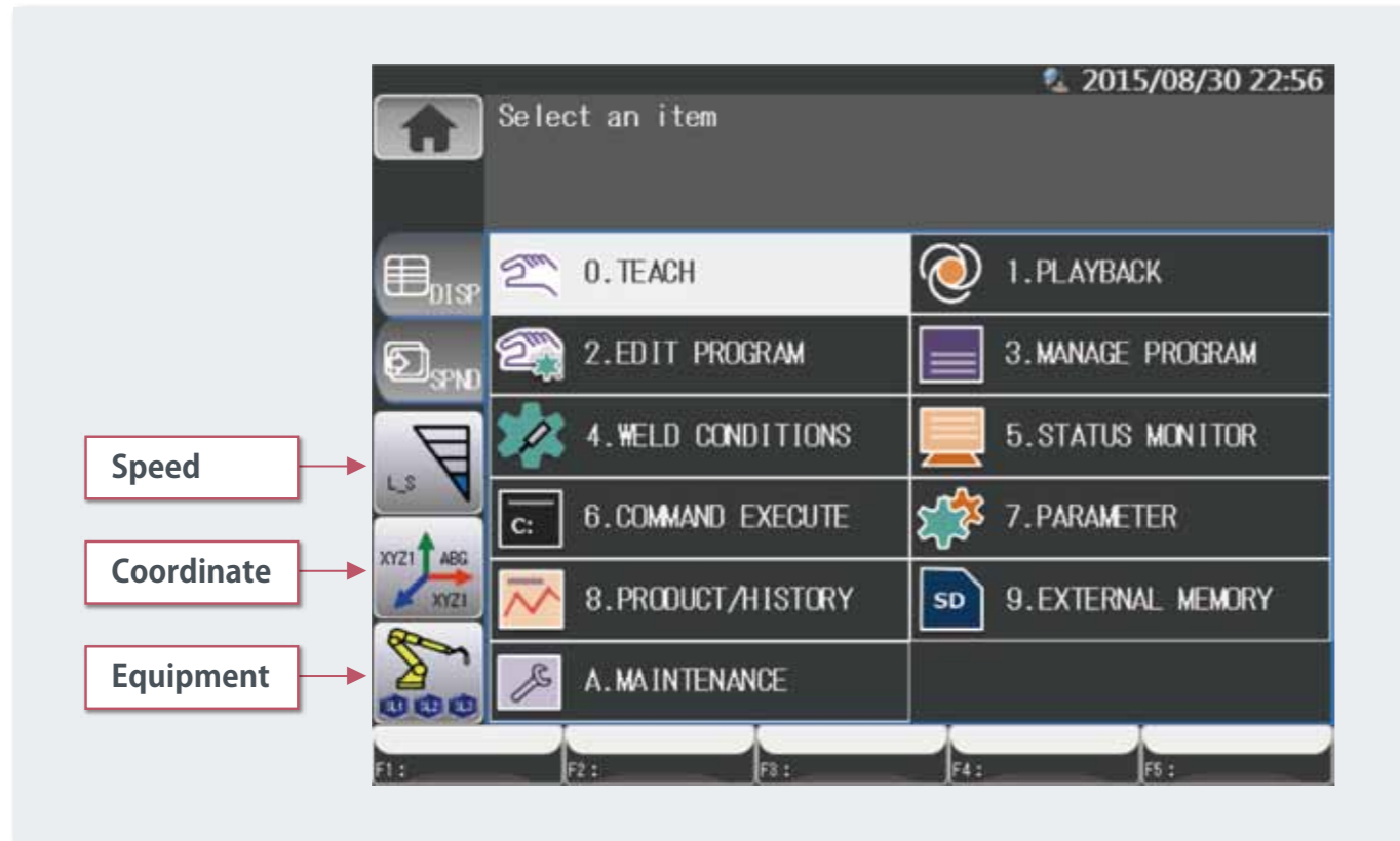
Figure 3 : Touch panel screen (upper part)
