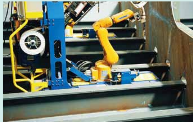
Figure 7: After lowered on to a bottom plate, the ARCMAN™ set fixes its position.
