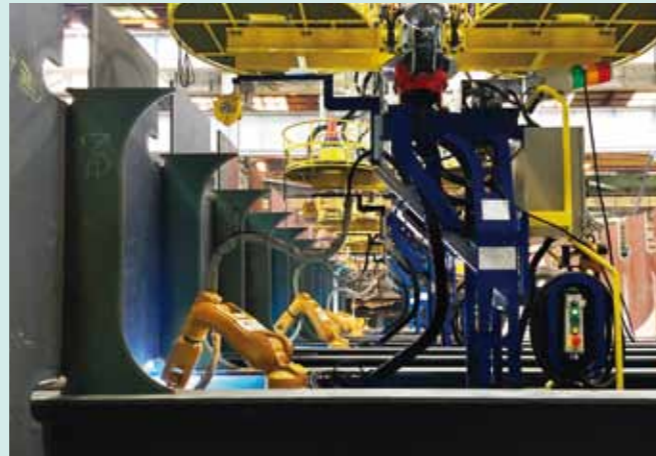
Figure 8: The ARCMAN™ set started welding.
