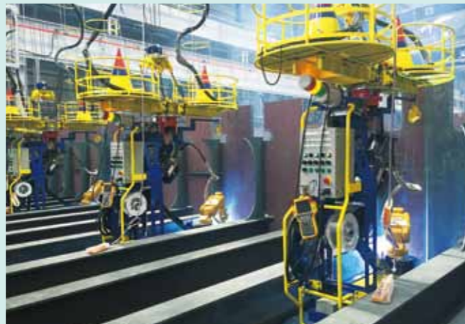
Figure 9: The ARCMAN™ set’s welding is in operation.
