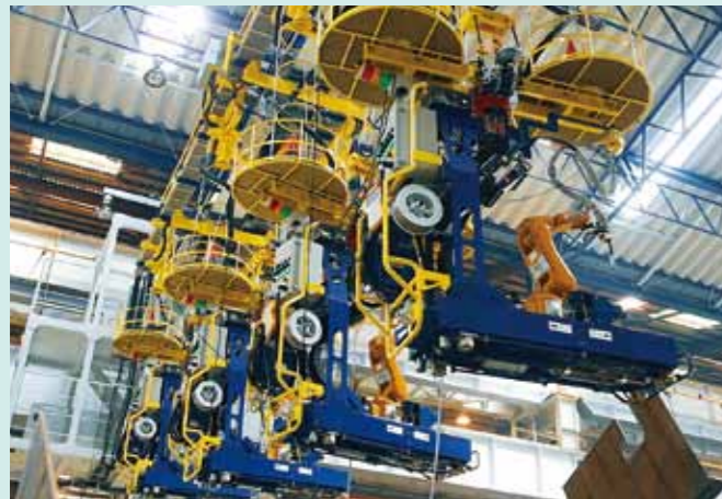
Figure 7: After lowered on to a bottom plate, the ARCMAN™ set fixes its position.
