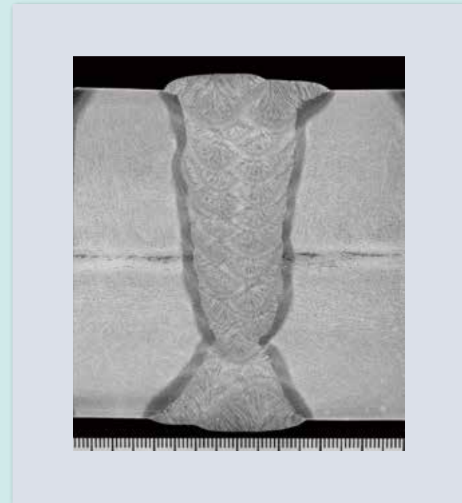
Figure 6: Macroscopic section of both side butt joint welding
