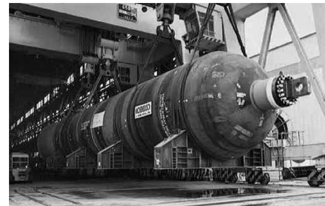
Hydro-desulfurization reactor is a typical pressure vessel for which temper embrittlement resistance is strictly required.
