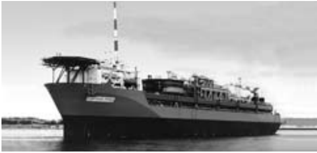
A floating production, storage and offloading vessel (FPSO). (Photo courtesy of Fene Shipyard, Italy)
