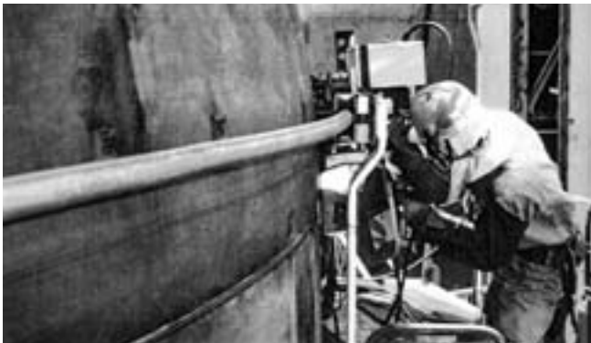
A typical application for DW-55LSR & DW-A55LSR – LPG tanks with a maximum plate thickness of 40 mm mounted on an LPG carrier requiring local stress relief heat treatment.
