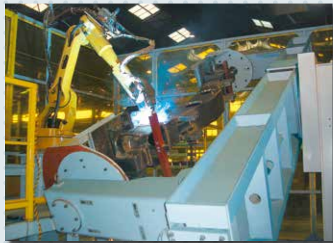
ARC MAN™ MP with drop-axis two-motion axis positioner (rotation and tilt)
