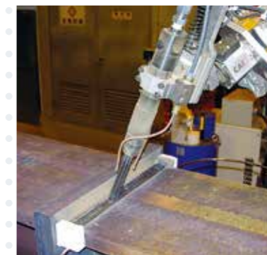
Automatic slag-removal device
