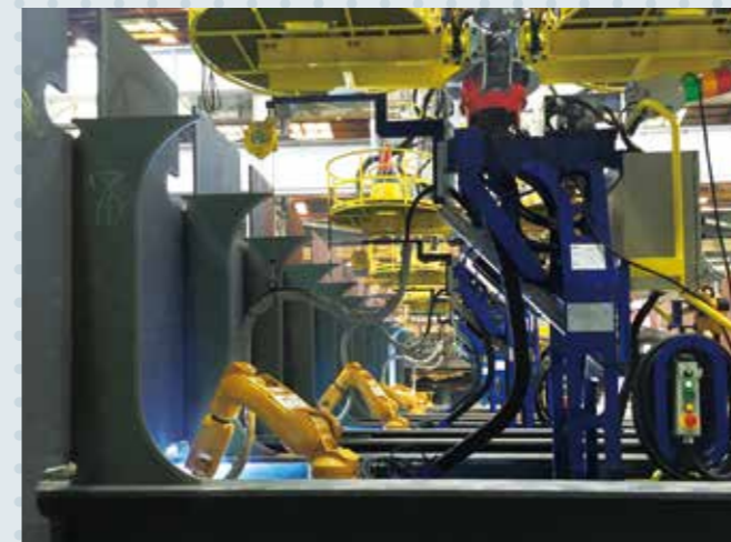
Large Assembly Welding System – ⑦
