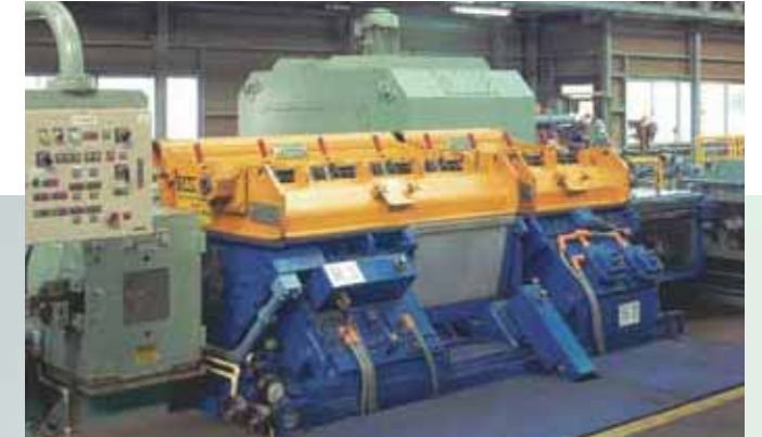
Sizing mill High-rigidity rolling mill capable of low-temperature rolling. This mill is capable of high dimensional accuracy rolling. (controlled rolling, dimensional control)
