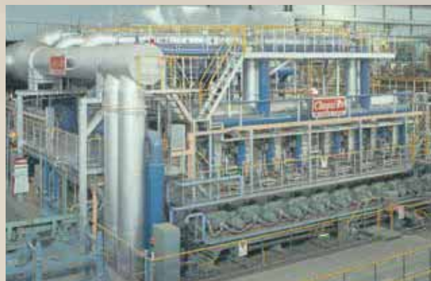
Heating furnace Billets are heated to about 1,000° C.
