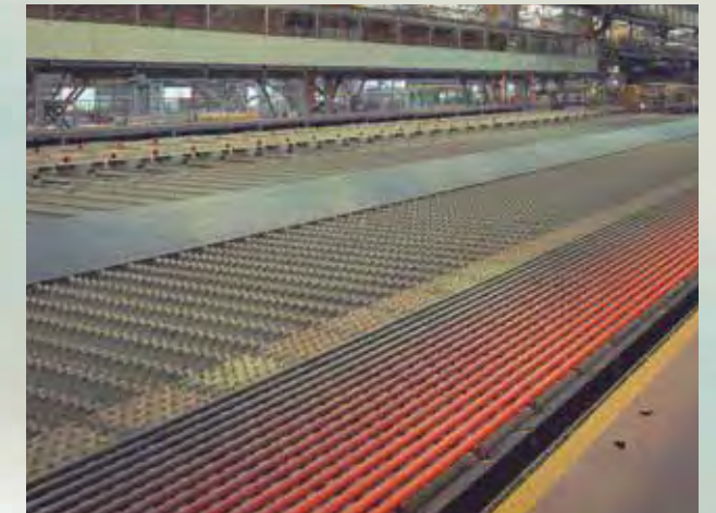
Cooling bed This cooling bed ensures uniform cooling for the entire length of the bars in order to minimize deflection.
