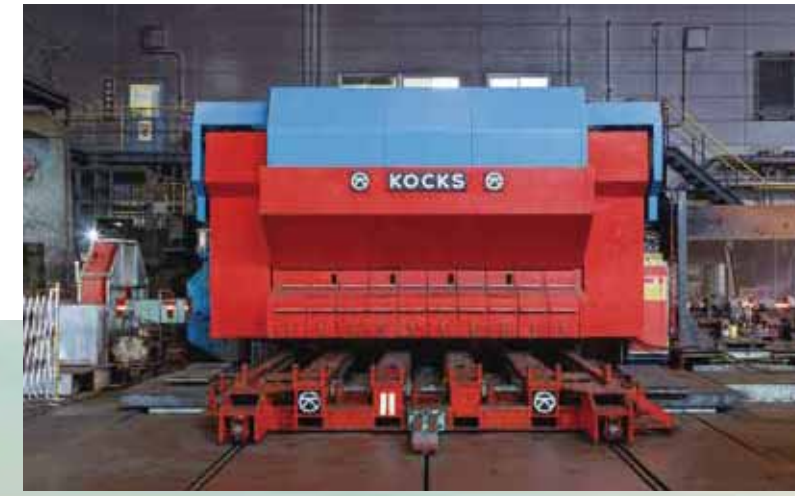
Block mill A three-roll system is adopted to assure high-precision rolling
