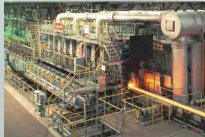
Heating furnace Billets are heated to about 1,000 °C
