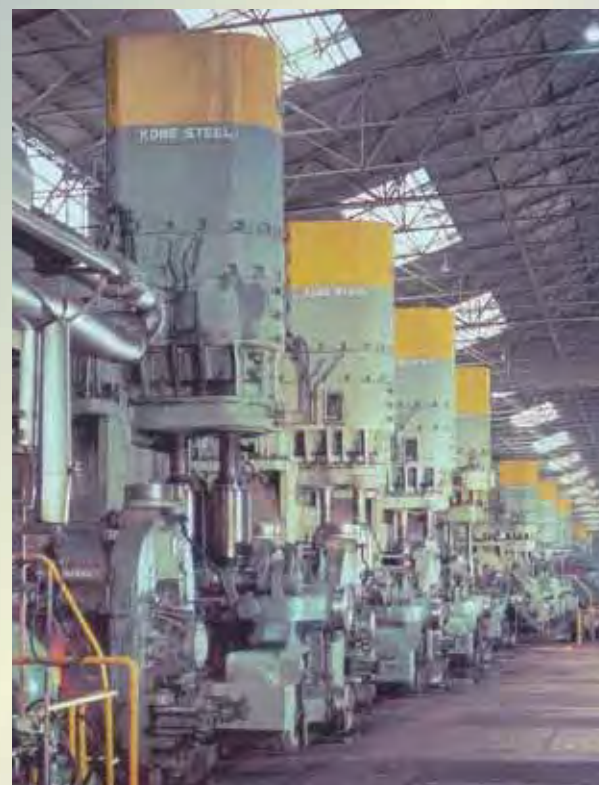
Roughing and intermediate trains Hot steel is passed through the grooved rolls to reduce its cross-sectional area.
