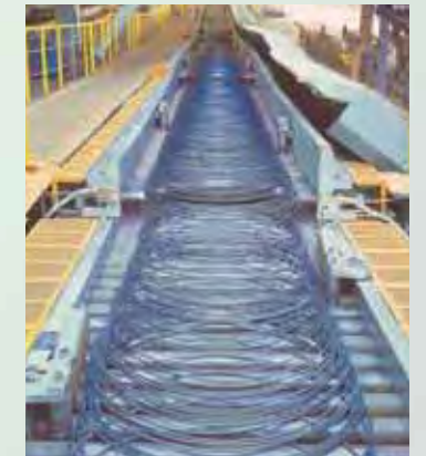
Product water cooling zone Rolling temperature is controlled (controlled rolling)
