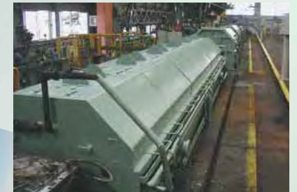
Product water cooling zone Rolling temperature is controlled (controlled rolling)
