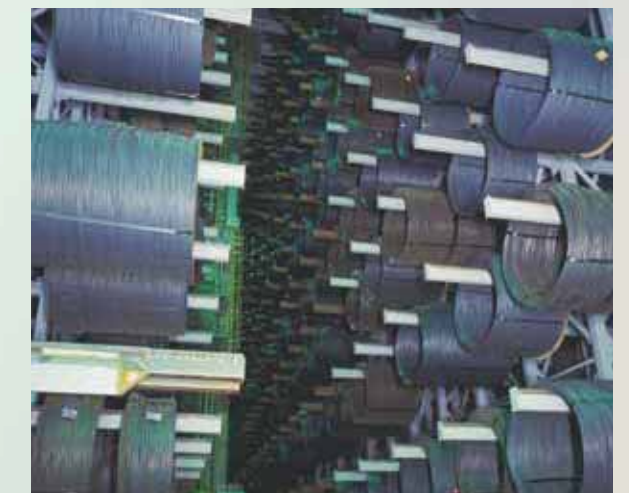
Automated warehouse After rolling, wire rods are unloaded from hook conveyor and directly stored in the automated warehouse.
