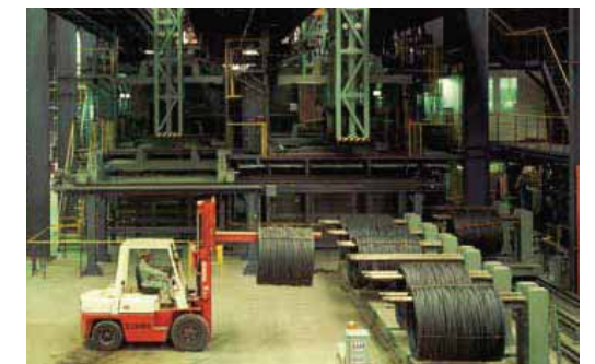
Automatic wire rod and coil pickling and coating facility
