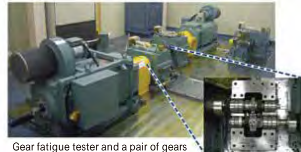
Gear fatigue tester and a pair of gears
