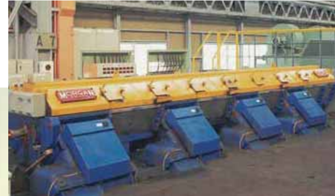
Finishing block mill High-rigidity rolling mill capable of low-temperature rolling. (controlled rolling)
