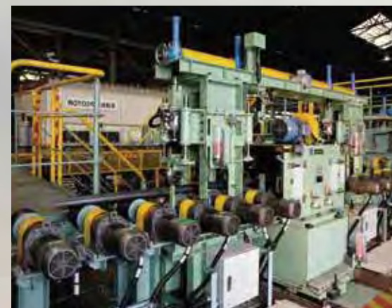
Magnetic leakage flux testing
