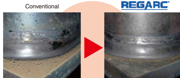
Comparison of the spatter attached to a diaphragm
